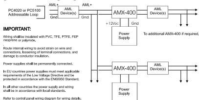
NOTE: Do not wire more than four AMX-400 modules in series from the source loop in series/parallel configurations
